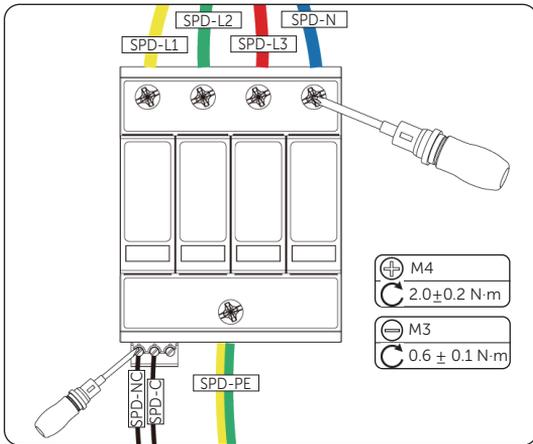
Figure 22-6 Connecting the SPD module cables
