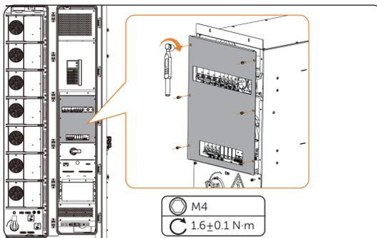
Figure 27-7 Mounting the panel
