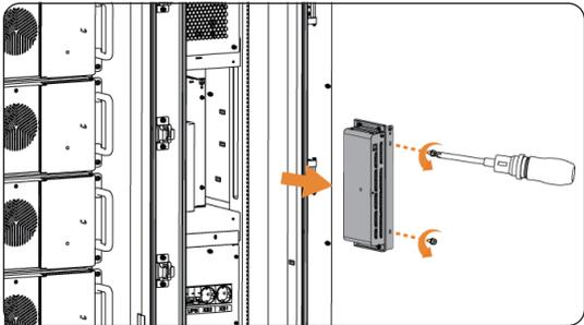
Figure 15-3 Removing the IO module
