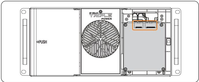
Figure 8-8 Connecting the cables of the BMU
