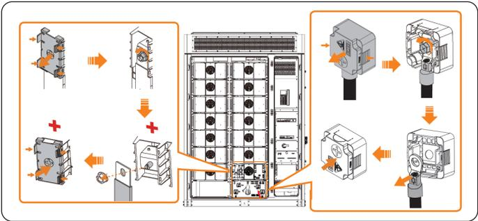
Figure 9-4 Removing the copper bars and cables
