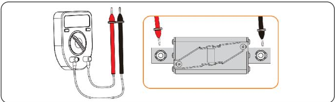
Figure 11-8 Measuring the fuse ON-OFF status
