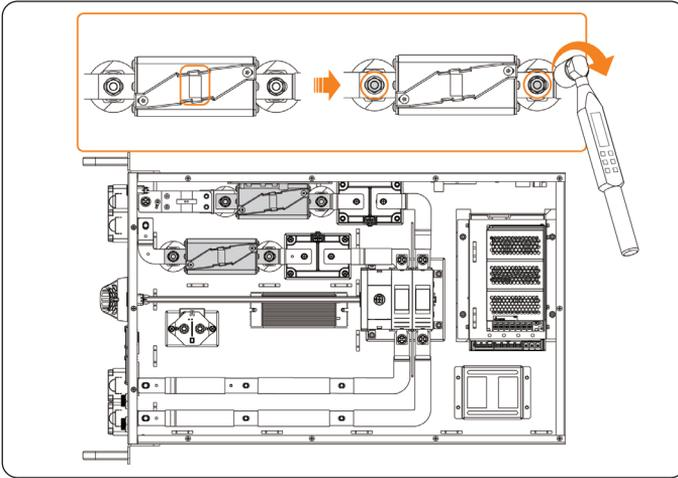
Figure 11-9 Removing the fuses (top view)
