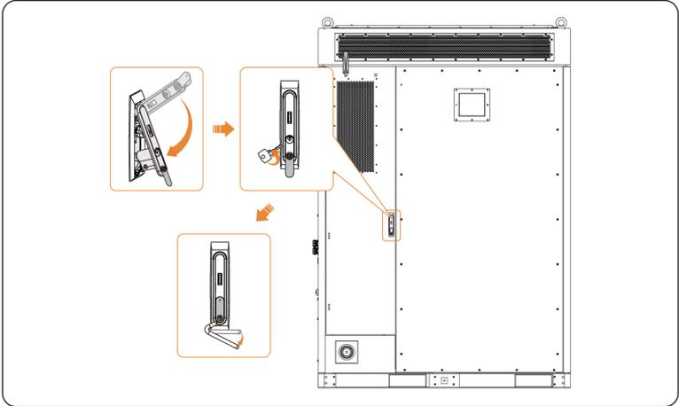
Figure 21-29 Closing the rear door
