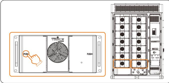
Figure 9-11 Closing the battery pack covers
