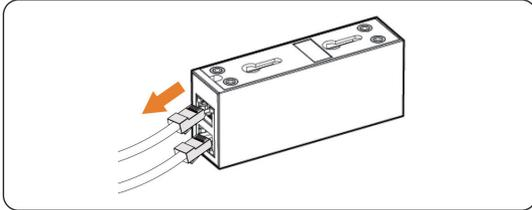
Figure 24-1 Removing cables
