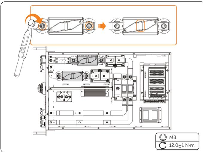
Figure 11-10 Installing the fuses (top view)
