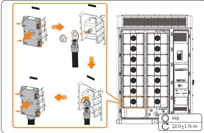
Figure 11-14 Connecting the negative power cable
