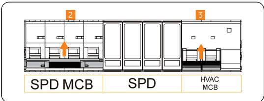
Figure 2-16 Flipping up breakers
