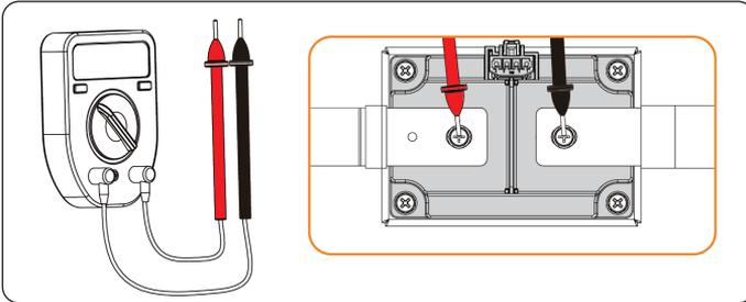
Figure 12-8 Measuring the contactor ON-OFF status
