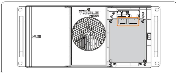
Figure 8-5 Removing the cables of the BMU
