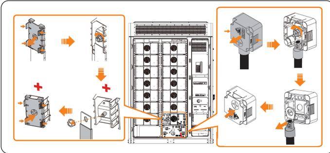
Figure 11-4 Removing the copper bars and cables
