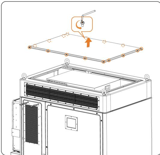
Figure 17-1 Remove the upper cover of the cabinet
