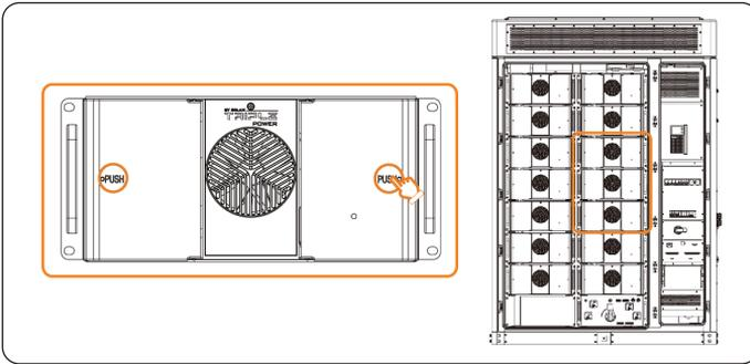
Figure 6-9 Closing battery pack covers
