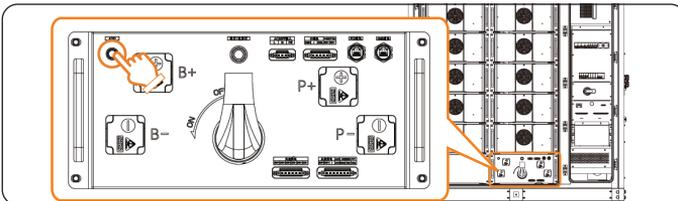
Figure 11-18 Address assignment
