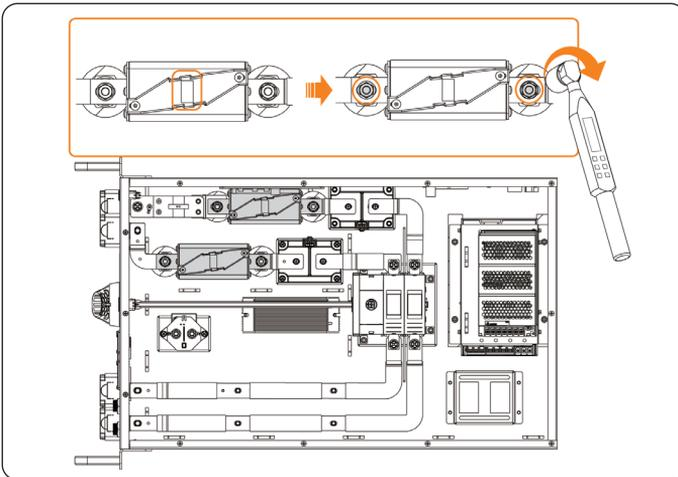
Figure 12-9 Removing the fuses (top view)
