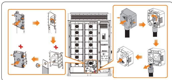
Figure 12-4 Removing the copper bars and cables
