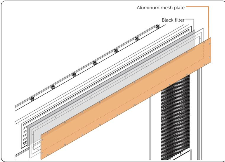
Figure 4-11 Dismantling aluminum mesh plate and black filter
