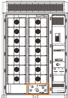
Figure 11-1 Position of the high-voltage box fuses
