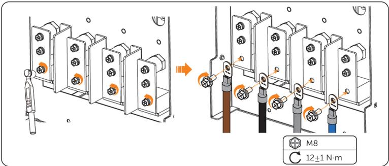
Figure 21-22 Connecting L1, L2, L3 and N cables
