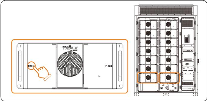
Figure 10-2 Opening the battery pack cover
