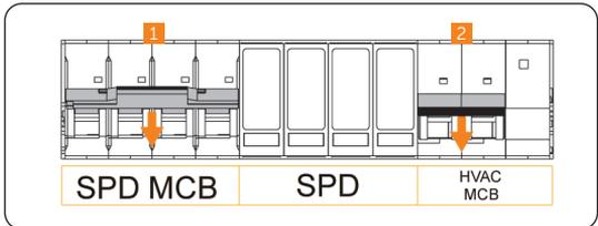
Figure 2-8 Flipping down breakers
