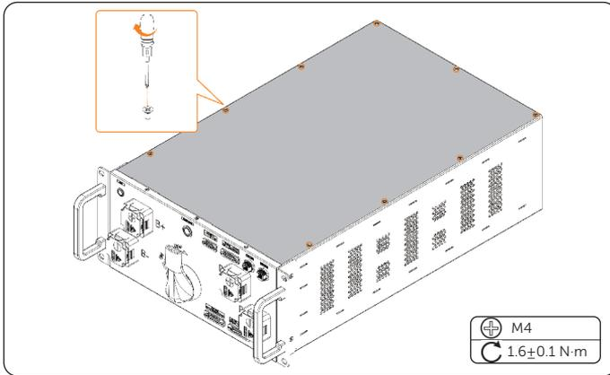
Figure 12-14 Installing the top cover
