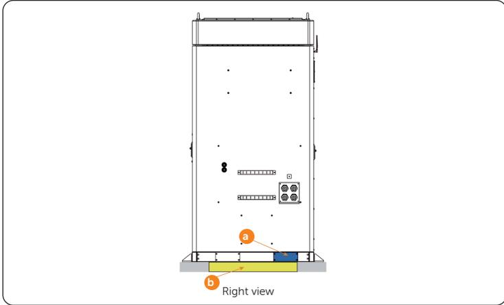
Figure 21-9 Pulling Grid cables out
