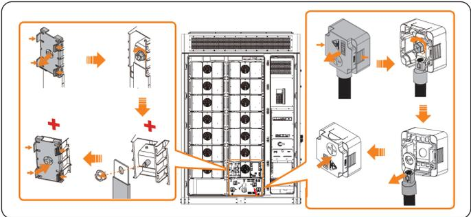
Figure 10-4 Removing the copper bars and cables
