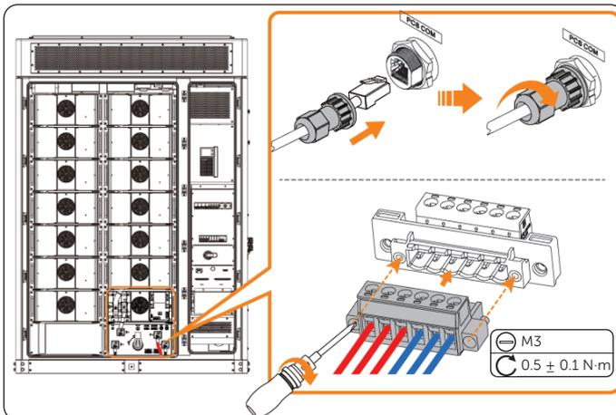
Figure 9-10 Connecting cables of high-voltage box
