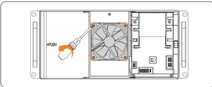
Figure 7-5 Removing the fan
