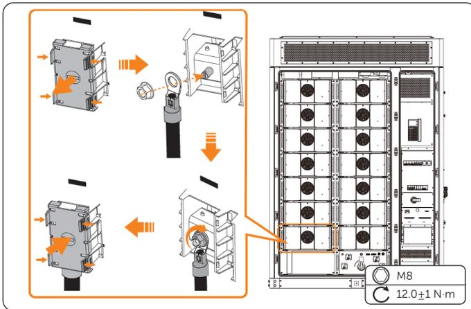
Figure 10-12 Connecting the negative power cable
