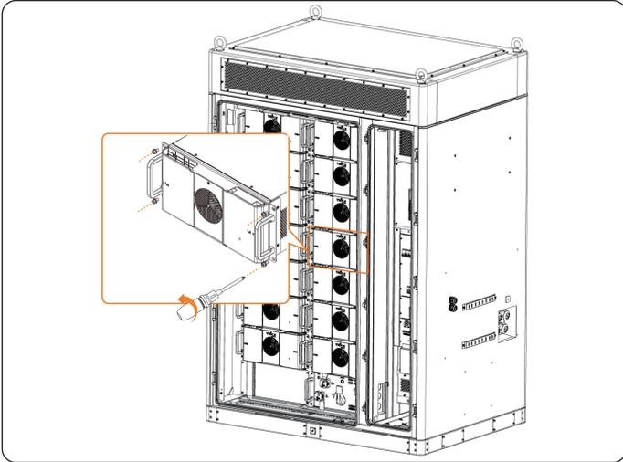
Figure 6-5 Removing screws on the battery pack
