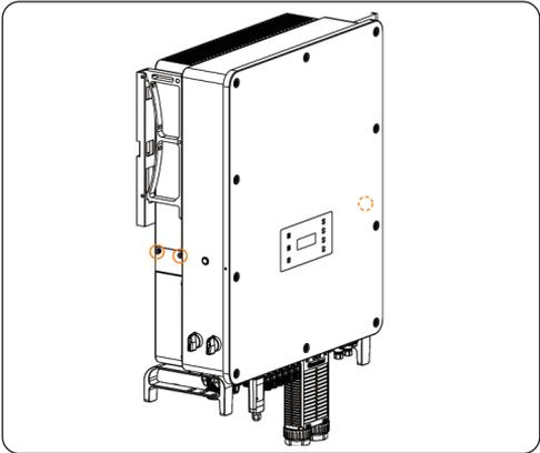
Figure 28-1 Dismantling screws
