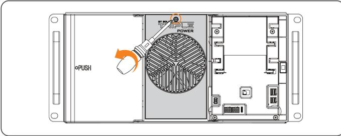
Figure 7-4 Removing the screw
