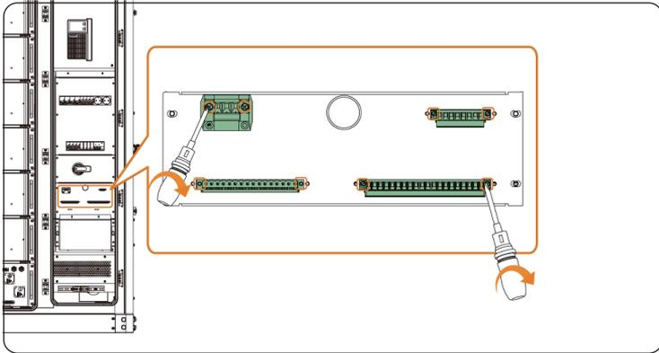
Figure 21-5 Removing the terminals
