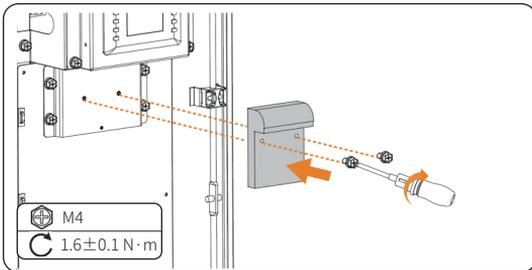
Figure 23-3 Installation of audible and visual alarm
