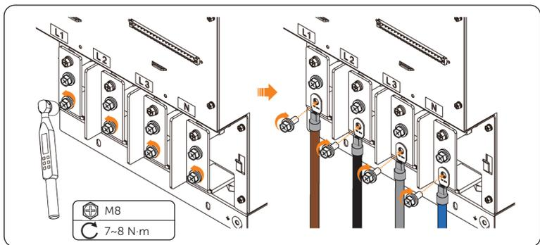
Figure 21-15 Connecting L1, L2, L3 and N cables
