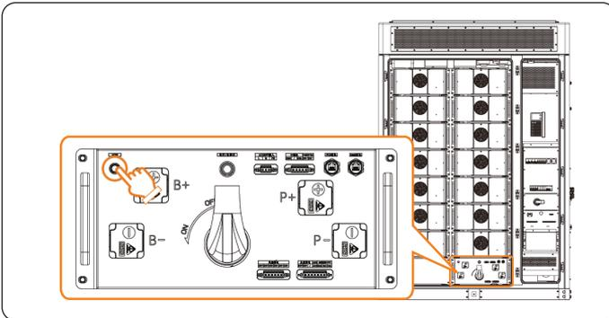
Figure 9-12 Address assignment
