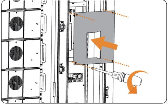
Figure 15-1 Removing panel
