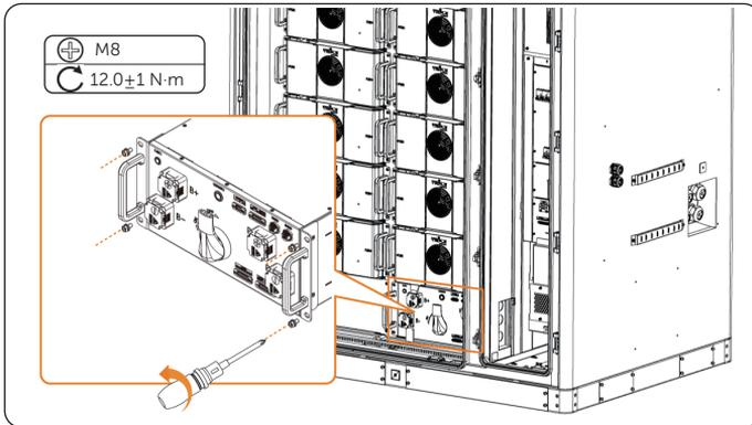
Figure 12-15 Installing the high-voltage box
