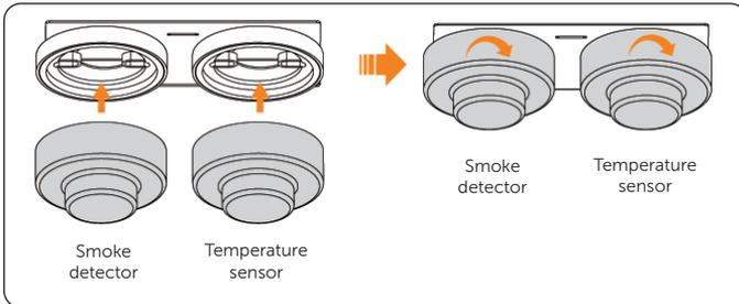
Figure 20-3 Installing the smoke detector and temperature sensor
