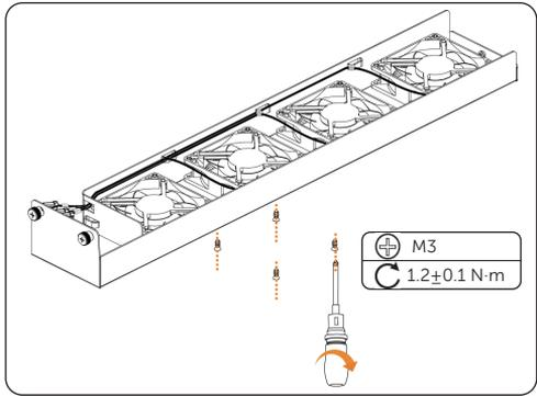
Figure 28-9 Lock the screws
