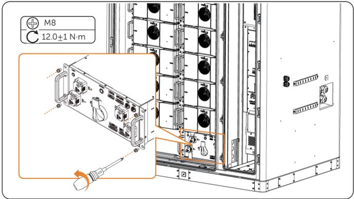
Figure 9-7 Installing the high-voltage box
