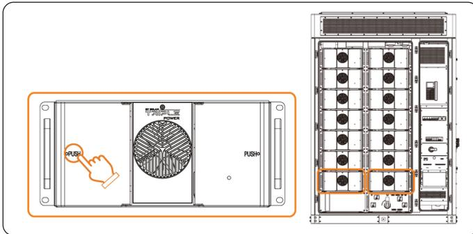
Figure 9-2 Opening the battery pack cover
