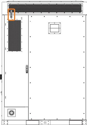
Figure 5-1 Position of the antenna (rear view)
