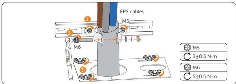
Figure 21-16 Tightening screws
