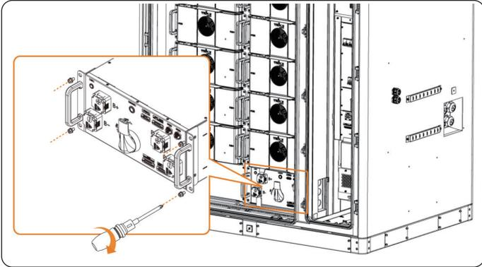
Figure 12-6 Removing screws on high-voltage box
