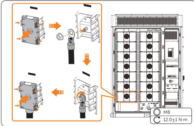
Figure 12-16 Connecting the negative power cable
