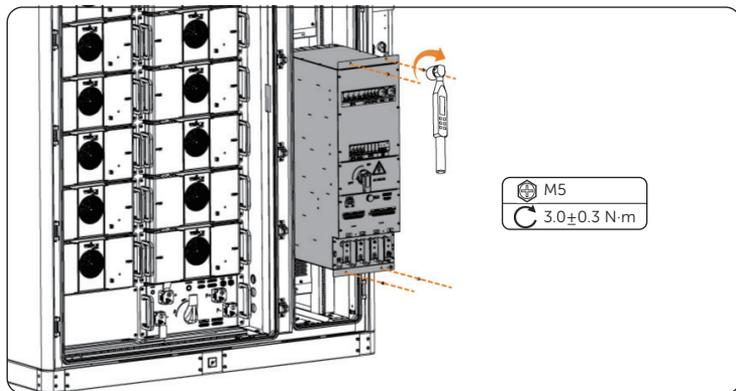
Figure 21-11 Installation of distribution box
