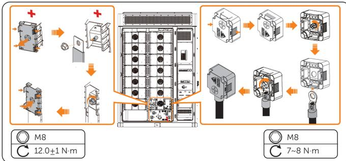
Figure 12-17 Connecting the copper bars and cables
