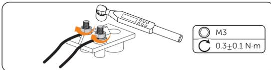
Figure 25-5 Connecting the cable
