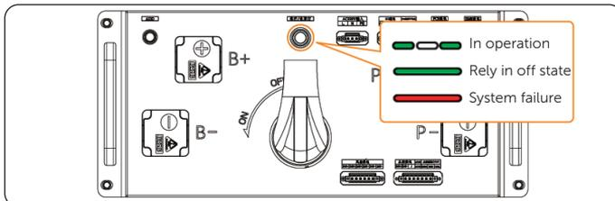
Figure 10-19 Checking the indicator
