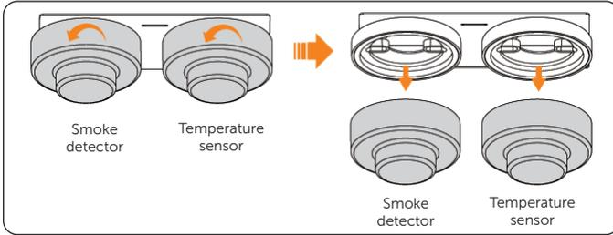
Figure 20-2 Removing the smoke detector and temperature sensor
