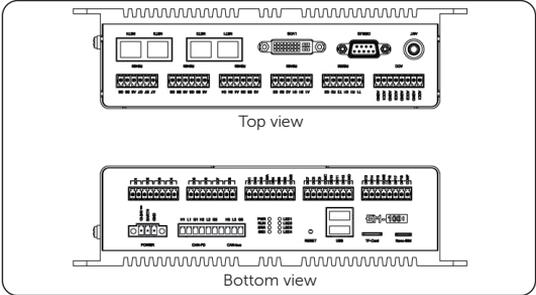
Figure 13-1 EMS1000 wiring area
