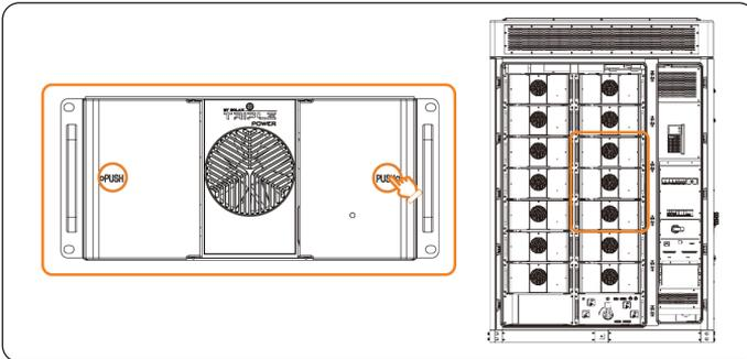
Figure 6-2 Opening the battery pack cover
