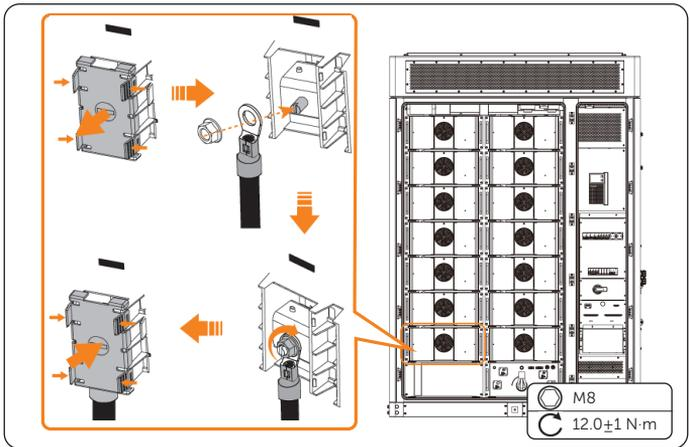
Figure 9-8 Connecting the negative power cable
