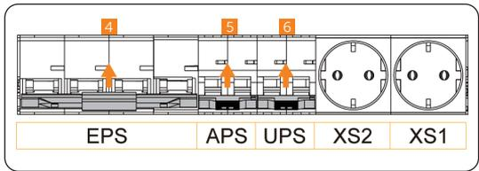
Figure 2-17 Flipping up breakers
