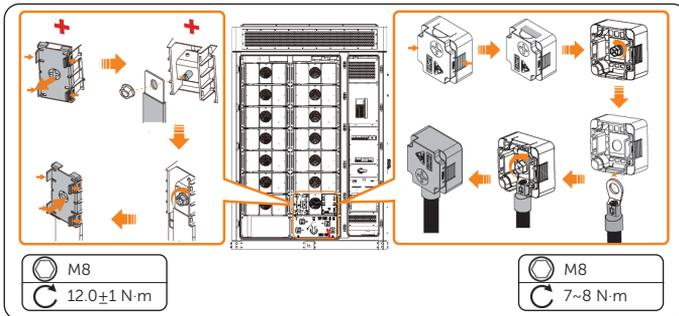
Figure 11-15 Connecting the copper bars and cables
