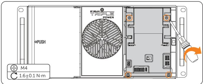
Figure 8-9 Installing the PCBA cover
