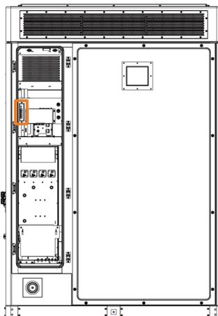
Figure 14-1 Position of the switch (rear view)
