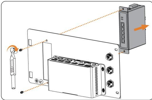
Figure 14-4 Removing the Switch from the sheet metal
