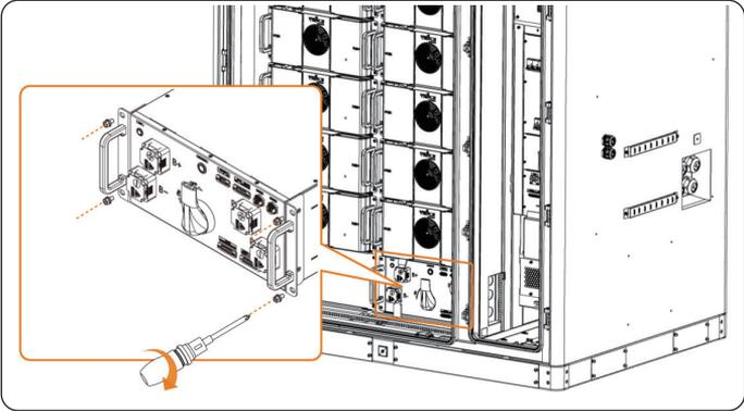
Figure 10-6 Removing screws on high-voltage box
