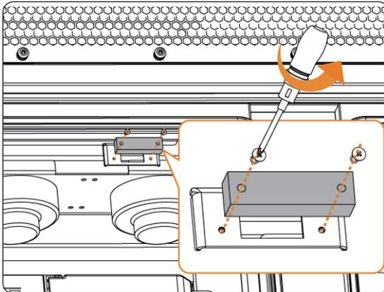
Figure 19-3 Removing the door sensor
