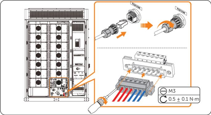
Figure 10-14 Connecting cables of high-voltage box
