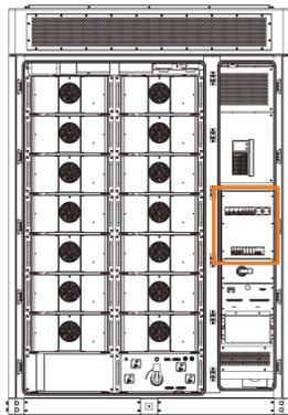
Figure 27-1 Position of UPS switch
