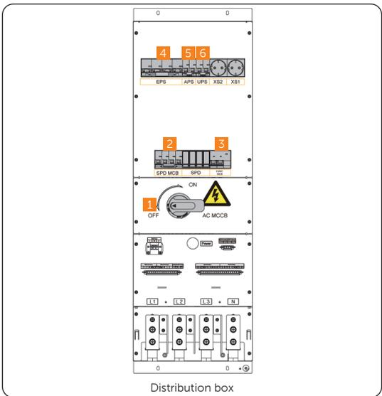
Figure 2-14 Starting sequence of distribution box
