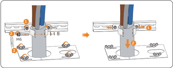
Figure 21-3 Removing the EPS cables
