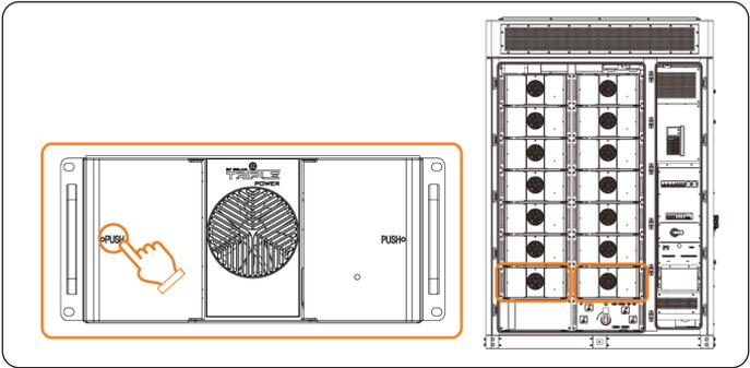
Figure 11-2 Opening the battery pack cover
