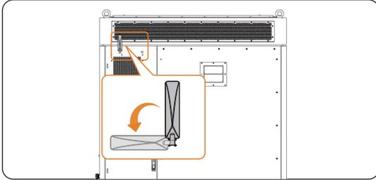
Figure 5-2 Removing antenna
