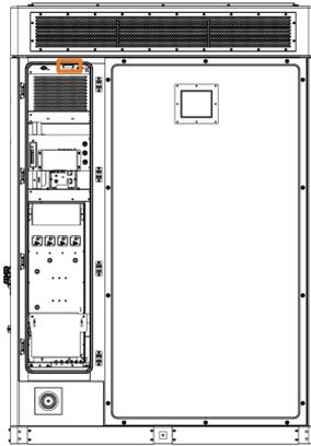
Figure 19-2 Position of the door sensor 3 (rear view)
