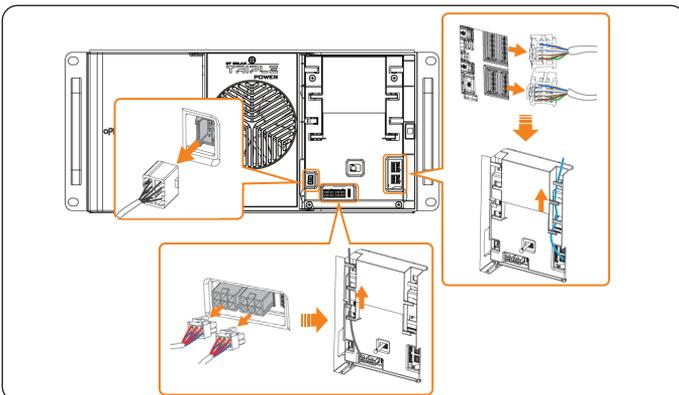
Figure 8-3 Removing the cables
