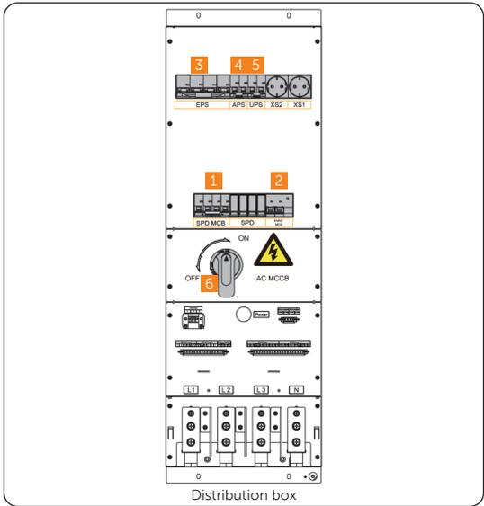
Figure 2-7 Shutting down sequence of distribution box
