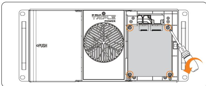
Figure 8-6 Removing the BMU
