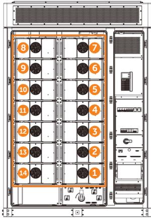
Figure 7-1 Position of the battery pack fans
