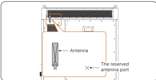
Figure 5-5 Well installed antenna
