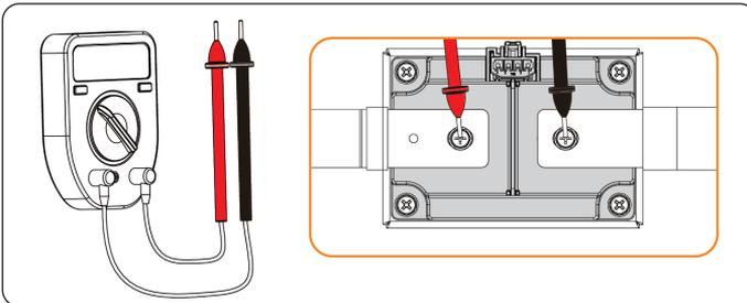
Figure 12-13 Measuring the contactor ON-OFF status
