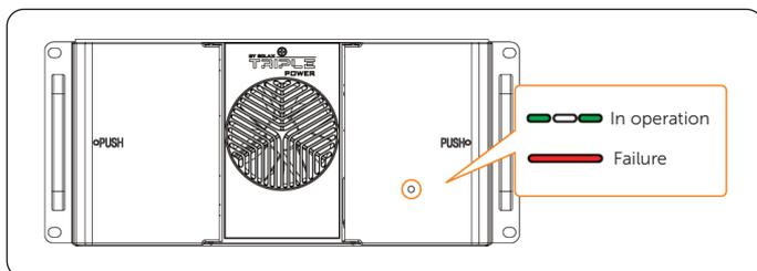
Figure 8-12 Battery pack indicator
