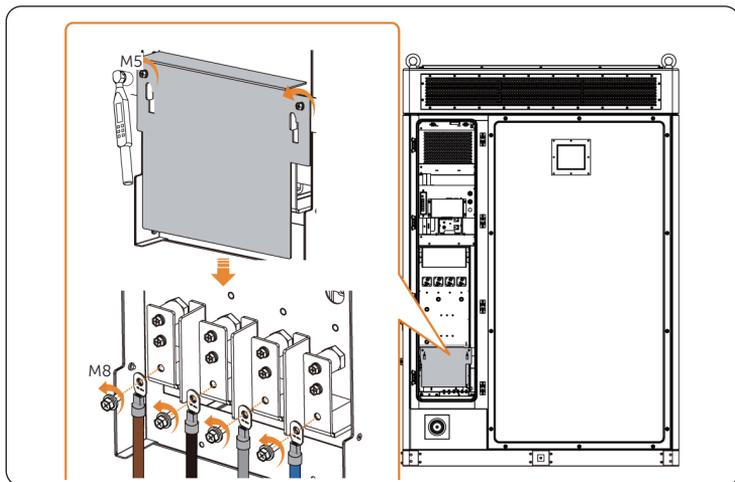
Figure 21-7 Disconnecting Grid cable
