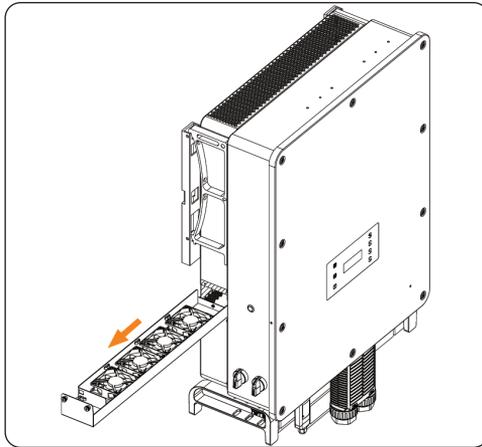
Figure 28-3 Pulling put the whole fan bracket
