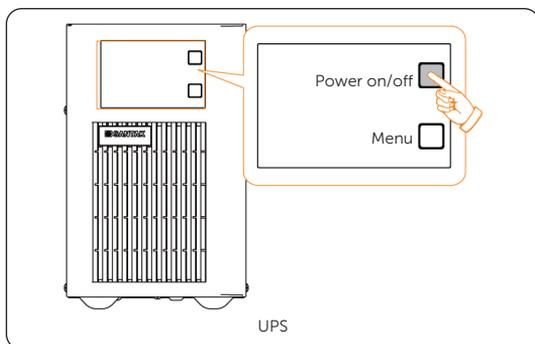
Figure 2-11 Holding and pressing button
