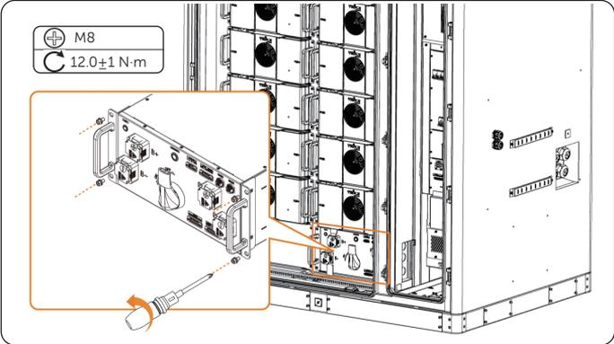
Figure 10-11 Installing the high-voltage box
