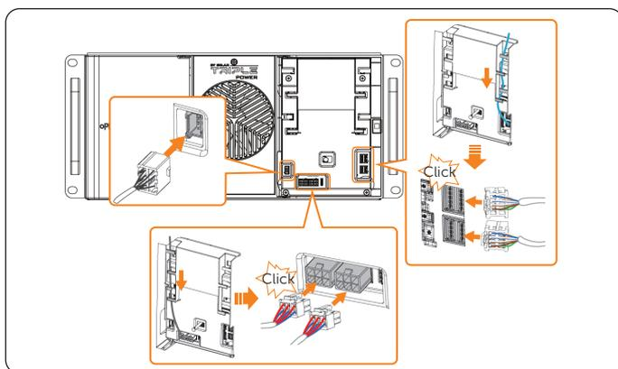
Figure 8-10 Connecting the cables of battery pack
