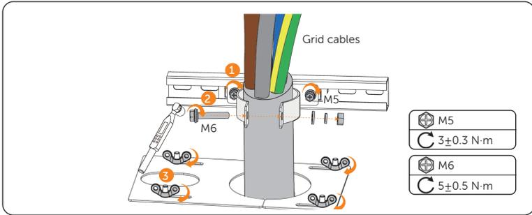
Figure 21-23 Tightening screws
