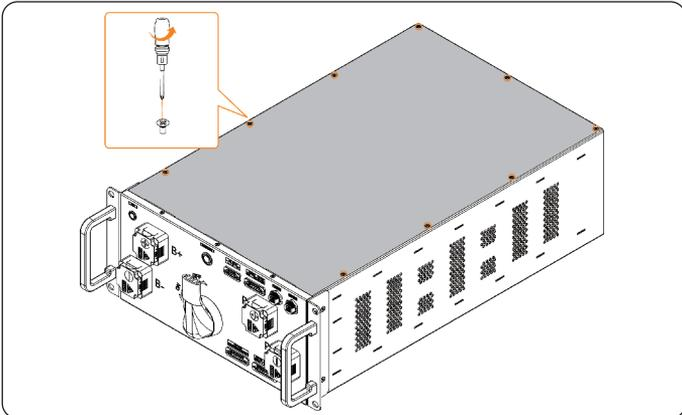
Figure 12-7 Removing the top cover
