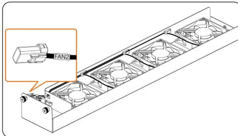
Figure 28-4 Identify the fan to be replaced
