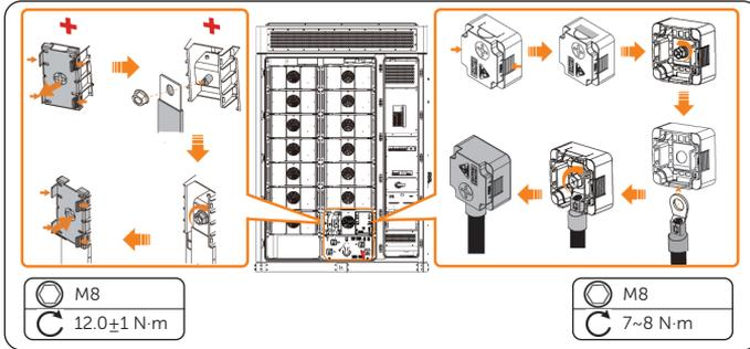
Figure 9-9 Connecting the copper bars and cables
