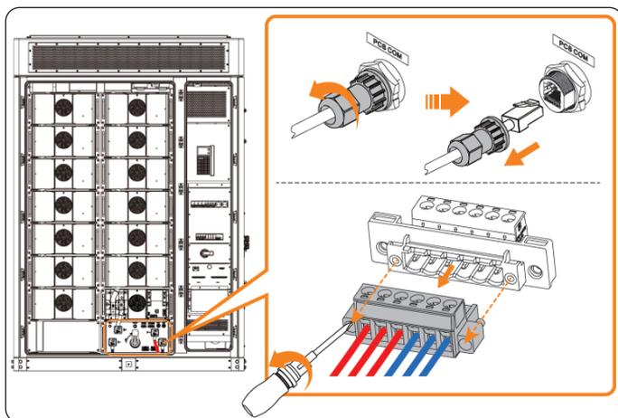
Figure 12-5 Removing cables of high-voltage box
