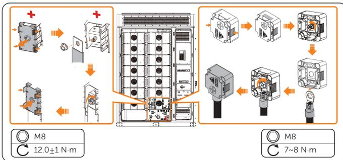
Figure 10-13 Connecting the copper bars and cables
