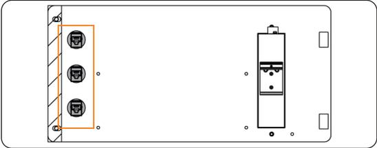
Figure 13-3 Sheet metal wiring area (rear view)
