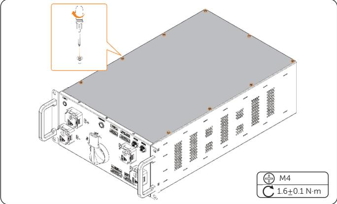
Figure 10-10 Installing the top cover
