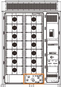
Figure 12-1 Position of the high-voltage box contactors
