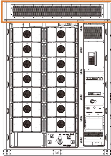
Figure 17-1 Position of the air conditioner
