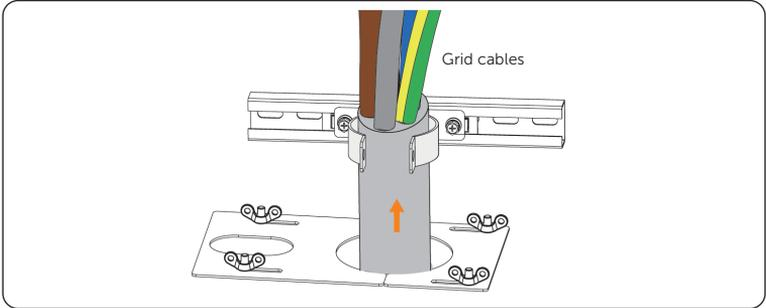
Figure 21-20 Threading grid cables
