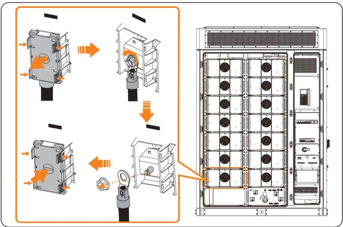
Figure 11-3 Removing the negative power cable
