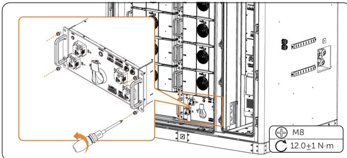
Figure 11-13 Installing the high-voltage box
