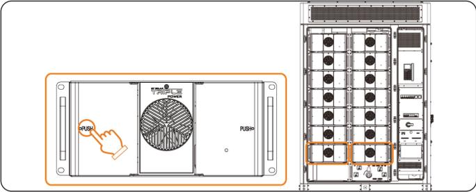
Figure 10-15 Closing the battery pack covers
