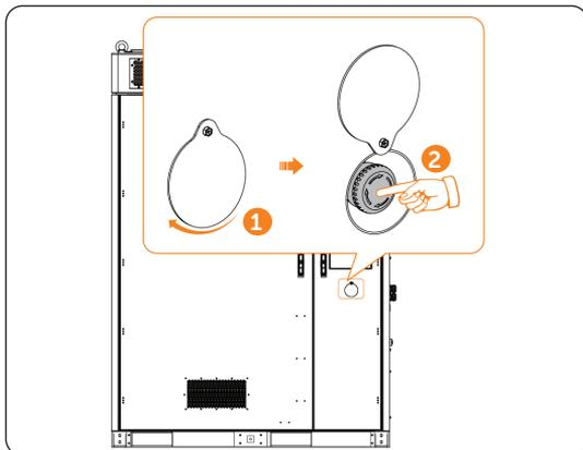
Figure 2-13 Pressing emergency stop button
