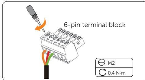
Figure 5-6 Securing wires
