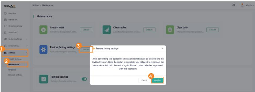
Figure 6-92 Restoring EMS1000 PRO to factory settings
