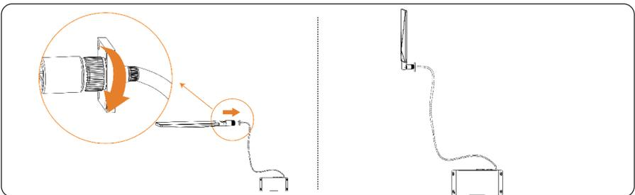
Figure 5-15 Fixing the antenna stick
