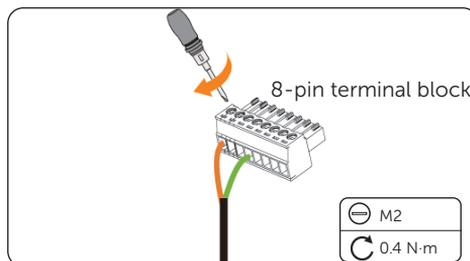
Figure 5-11 Securing wires
