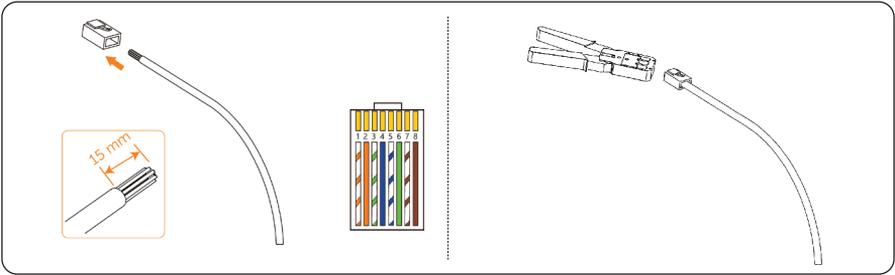
Figure 5-2 Stripping and crimping network cable
