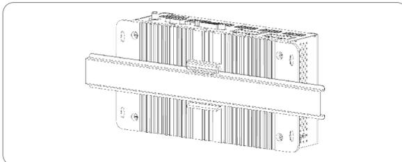
Figure 4-2 Clasping the DIN rail buckle to rail
