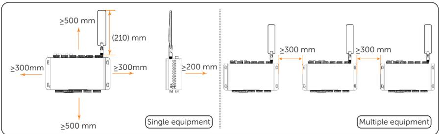
Figure 3-3 Clearance requirements
