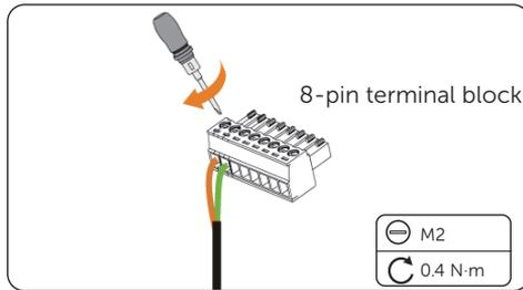
Figure 5-8 Securing wires
