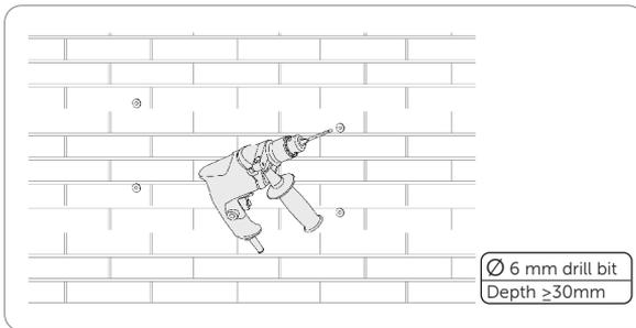
Figure 4-4 Drilling holes
