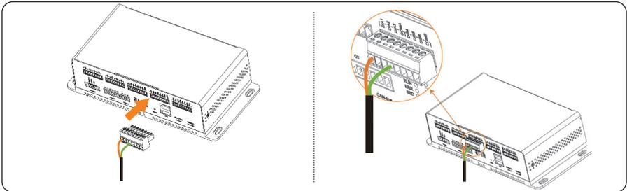
Figure 5-12 Inserting the terminal block
